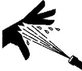
**WARNING:** The fluid supply system on which this applicator is used may be pressurized! Relieve system fluid pressure before breaking any connection. Failure to relieve the system fluid pressure can result in the uncontrolled release of fluid that can cause personal injury, including death.
